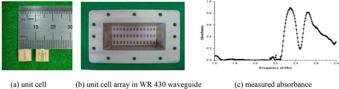
Fig. 3: Photographs of the fabricated absorbers and experimental results of unit cell array.
