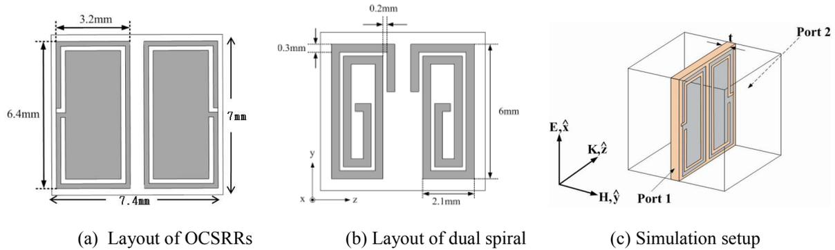
Fig. 1: Schematics of optimum single-cell absorber and simulation setup.
