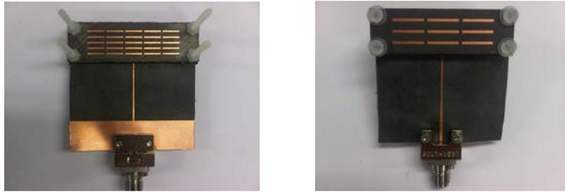
Fig. 3. Top and back views of the dual-band dipole with meta-surfaces.
