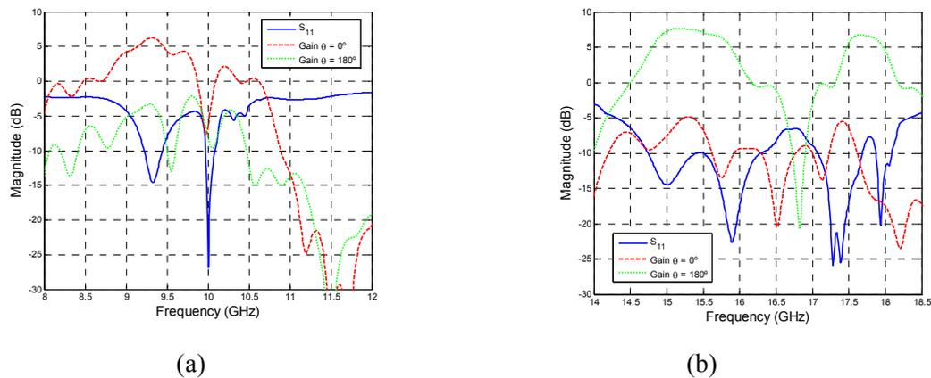
Fig. 4. Measured antenna performance in the (a) low and (b) high frequency bands.
