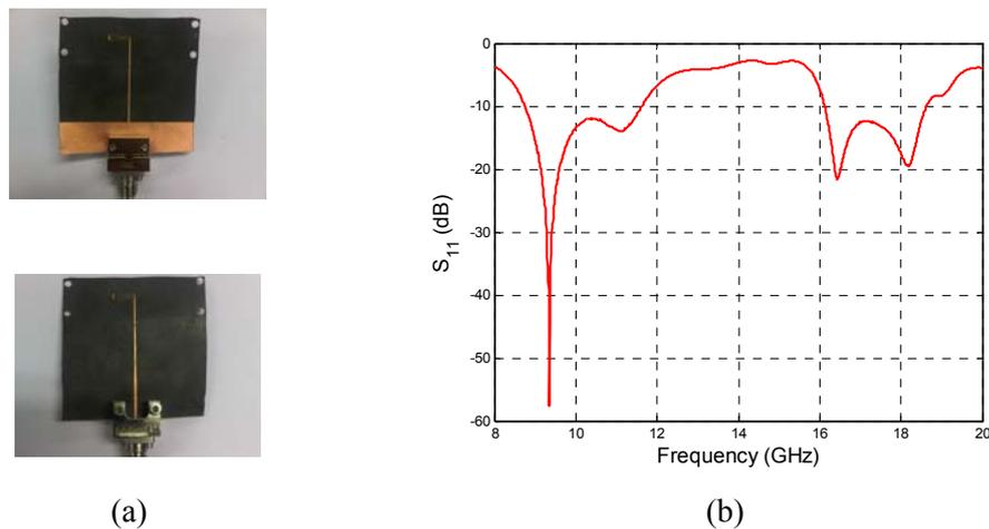
Fig. 2. (a) Top and back views of the dual-band dipole. (b) Measured antenna return loss.
