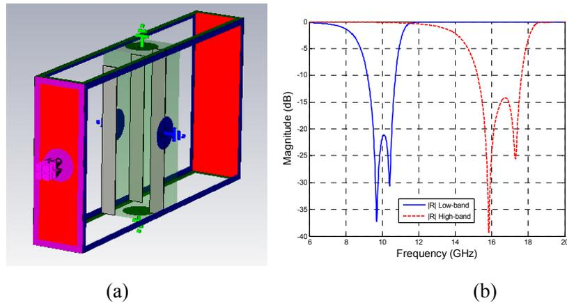
Fig. 1. (a) Unit cell CST model. (b) Simulated reflection coefficients for the low-band and high-frequency band meta-surfaces.
