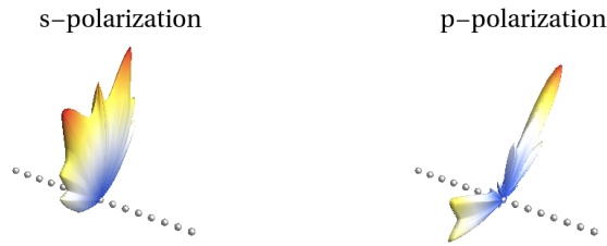
Fig. 3: Emission pattern for s -polarized (left) or p -polarized (right) excitation at \theta = 35^\circ and \phi = 90^\circ .
