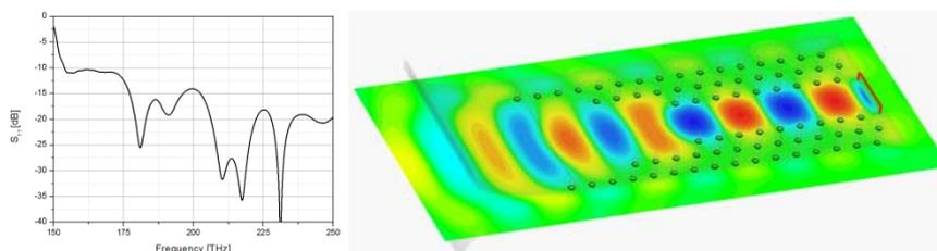
Fig. 2: (a) Amplitude of the scattering parameter  $S_{11}$  at the input port of the horn nano-antenna reported in Fig. 1 as a function of frequency. (b) Map of the electric field amplitude distribution at the design wavelength of  $1.5 \mu\text{m}$ .
