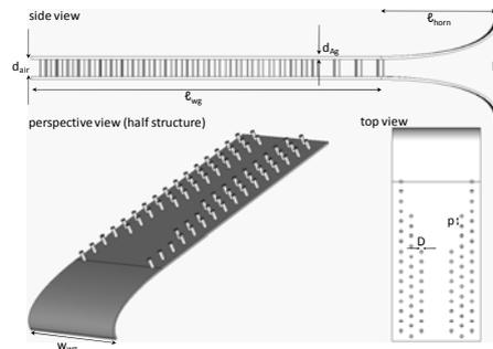
Fig. 1: Horn nano-antenna geometry.  $l_{wg} = 6 \mu\text{m}$ ,  $l_{horn} = 2 \mu\text{m}$ ,  $h = 2 \mu\text{m}$ ,  $w_{wg} = 3,25 \mu\text{m}$ ,  $d_{air} = 300 \text{ nm}$ ,  $d_{Ag} = 50 \text{ nm}$ ,  $D = 100 \text{ nm}$ ,  $p = 375 \text{ nm}$ .
