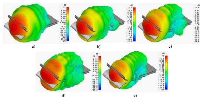
Fig. 3: 3D gain radiation pattern of the horn nano-antenna reported in Fig. 2 at a)  $160 \text{ THz}$ , b)  $180 \text{ THz}$ , c)  $200 \text{ THz}$ , d)  $220 \text{ THz}$ , and e)  $240 \text{ THz}$ .
