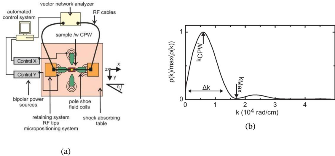
Fig. 1: (a) Sketch of the probe station with VNA and field coils. (b) Normalized Fourier transformation of the current density distribution of a coplanar waveguide having an inner conductor width of 2  $\mu\text{m}$ .
