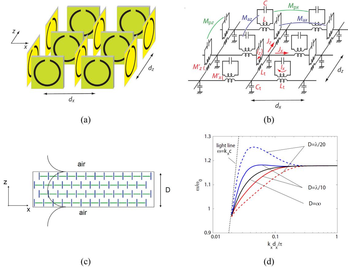
Fig. 1: (a) A metamaterial consisting of two sub-lattices of split rings; (b) its equivalent circuit model; (c) top view of a slab of a brick-wall SRR metamaterial; (d) surface proxiton-polariton dispersion for various thicknesses  $D$  of the brick-wall slab.  $\kappa_{ax} = 0.1$ ,  $\kappa_{px} = 0.1$ ,  $\kappa_{az} = \kappa_{pz} = 0$ ,  $q_x^2 = q_z^2 = 0.56$ ,  $d_x = d_z = \lambda/100$ .
