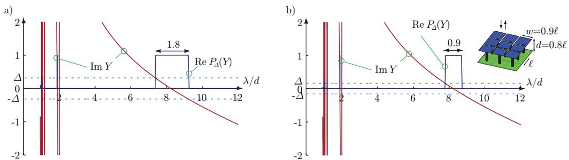
Fig. 2: Normalized admittance  $Y$  and composition  $P_\Delta(Y)$  with  $\Delta = \{1/\pi, 1/(2\pi)\}$  for a mushroom structure with  $\ell = 10$  mm,  $w = 9$  mm, and  $d = 8$  mm. a)  $\Delta = 1/\pi$  with the lossless bound  $\lambda_2 - \lambda_1 \leq 2$ . b)  $\Delta = 1/(2\pi)$  with the lossless bound  $\lambda_2 - \lambda_1 \leq 1$ .
