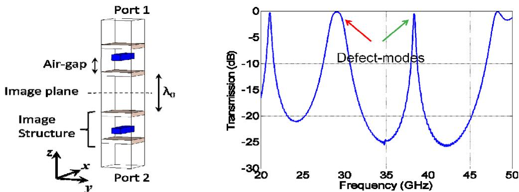
Fig. 2: Unit-cell model and its transmission factor for normal incidence.
