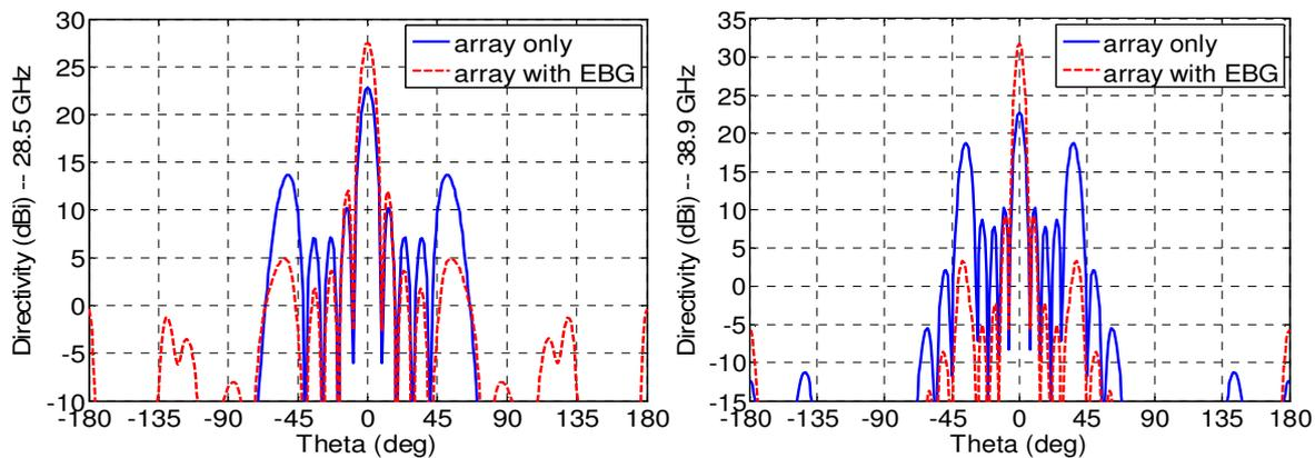
Fig. 4: Grating lobe suppression in EBG resonator antenna excited with an array feed.
