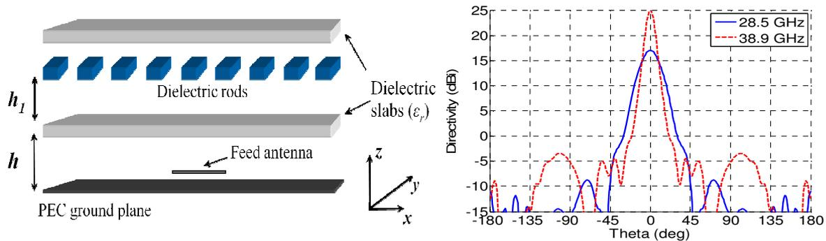
Fig. 1: Dual-band EBG resonator antenna configuration and peak directivities.
