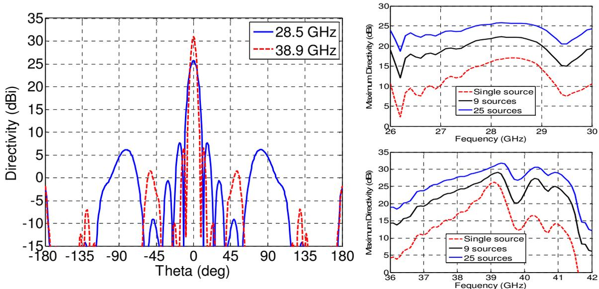
Fig. 3: Computed  $E$ -plane radiation patterns and radiation bandwidth with 25 HED sources.
