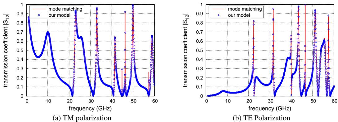
Fig. 2: Transmission spectra for a structure with parameters:  $a = 5.0$  mm,  $d_1 = 2.0$  mm,  $d_2 = 3.0$  mm,  $\varepsilon_1 = 2.2$ ,  $\varepsilon_2 = 3.0$ ,  $w = 0.5$  mm.
