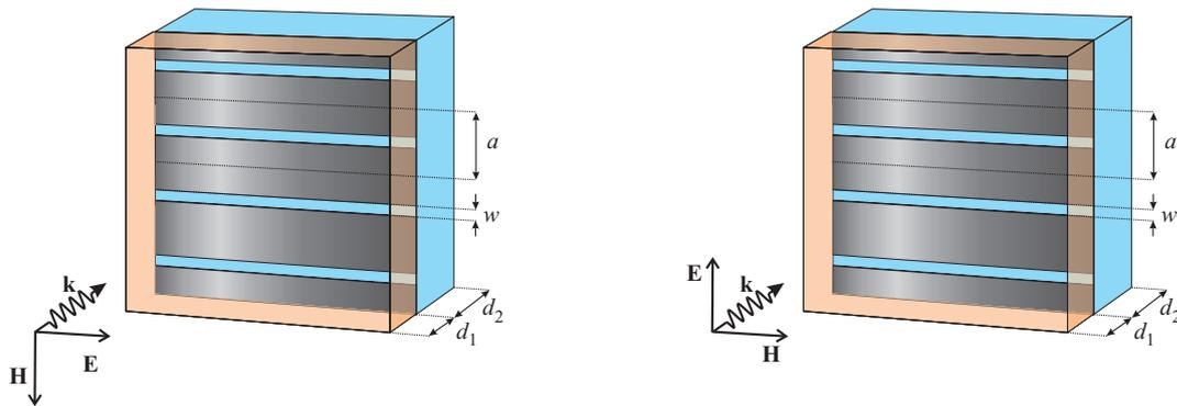
Fig. 1: Example of structure under consideration under normal TM and TE illumination. Narrow strips and oblique incidence have also been considered.
