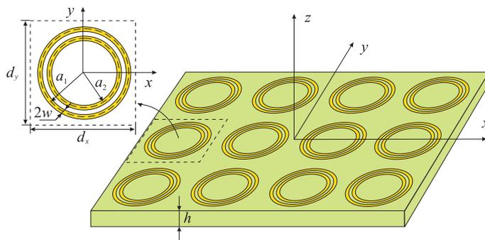
Fig. 1: Fragment of the planar metamaterial and its elementary unit cell.
