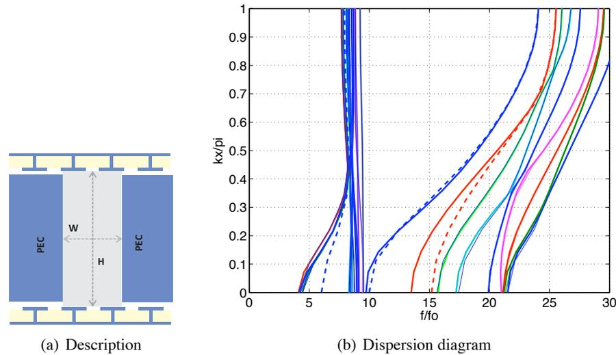
Fig. 3: Waveguide designed with the double mushroom-EBG surfaces. Aperture size is 5mmx5mm for solid lines and 5mmx3mm for dashed lines.
