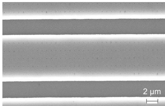
Fig. 1: Scanning electron microscopy picture showing a coplanar wave guide (bright color) on top of a permalloy film (dark) where parts of the film are patterned with a periodic array of holes. Their diameter amounts to 120 nm.
