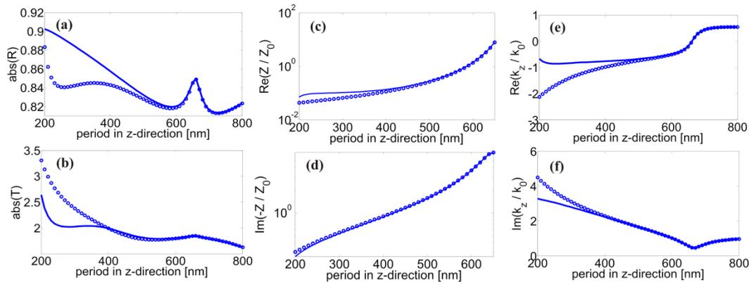
Fig. 1: (a),(b) Scattering coefficients at the single interface. Solid lines represent rigorous results and symbols are calculated using Eqs. (4). In figures (c)-(f) the solid lines are achieved using the properties of the fundamental Bloch mode of the swiss-cross MM. The symbols are those results achieved by a parameter retrieval procedure of the associated single layer slab MM.
