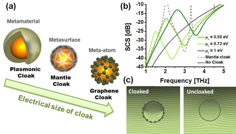
Fig. 2: (a) Evolution of scattering-cancellation-based cloaks. (b) Total SCS of a dielectric sphere with diameter  $D = \lambda_0 / 5$  and  $\epsilon_d = 5$ , with (1) lossless mantle cloak ( $X_s = 222.5 \Omega$ ) (gray dash), (2) graphene cloak with different chemical potential (green), and (3) without (gray solid) cloak. (c) Uniform phase distribution of H field on the E plane for the graphene-coated object at the frequency of operation, compared with the uncoated one.
