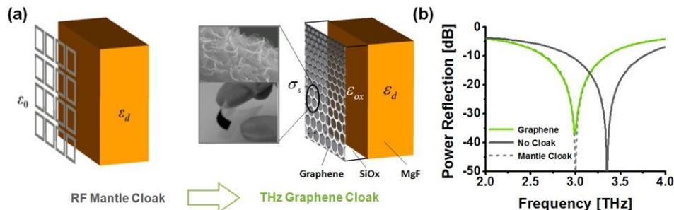
Fig. 1: (a) Illustration of a graphene cloak (the inset shows graphene flakes obtained using MPCVD). (b) Power reflection for a  $\lambda_0/5$ -slab of MgF or KBr ( $\epsilon_d \sim 5$ ) (1) with ideal mantle cloak  $X_s = 1248\Omega$  (gray dashed), (2) with graphene on a  $1.56\mu\text{m}$   $\text{SiO}_2$  film (green dashed), and (3) without cloak (gray solid).
