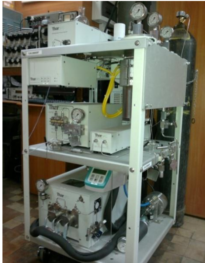
Fig.1. Supercritical fluid extraction unit SFE - 1000.
