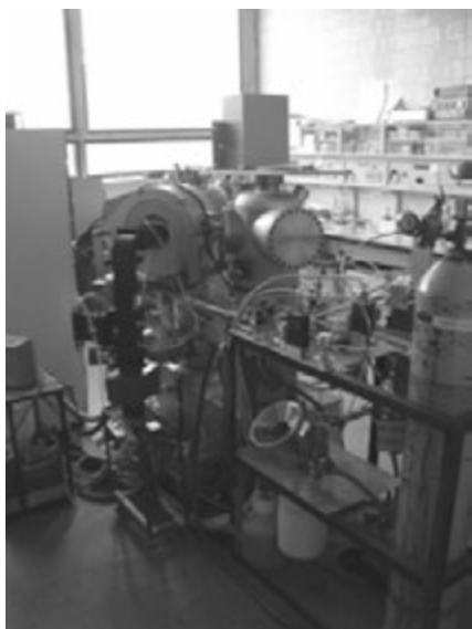
Fig. 1. The experimental EpiLab 150 setup used for layers growing.
