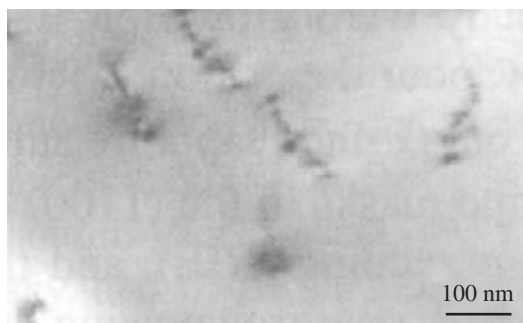
Fig. 3. TEM view of dislocation domain boundaries after degradation
