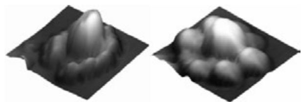
Fig. 1. AFM image of grown nanostructure. Inserted enlarged 3D AFM images are the typical structures for the given sample. Figure is 5 \times 5 \mu\text{m} , insertions are 530 \times 530 \text{ nm} .
