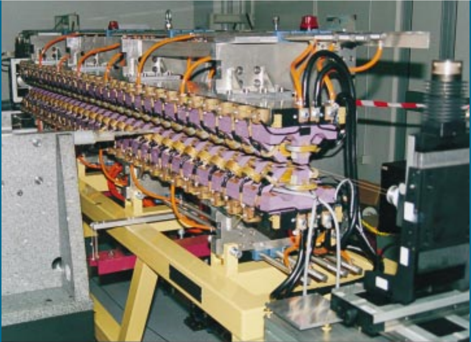
Fig. 13: The latest addition to ELETTRA's insertion devices: the electromagnetic elliptical wiggler.
