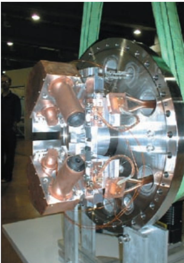
Figure 1: The New PBPM prototype layout. The flange of the manipulator supports the detector. The main active elements are visible: the blades, that intercept the photon beam, and the hemispherical analysers that collect and filter the photoemitted electrons.
