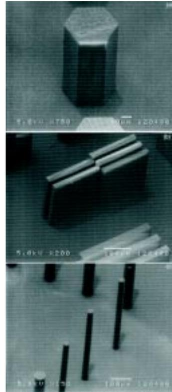
**Figure 2.** Examples of high aspect ratio PMMA test microstructures produced at ELETTRA.
