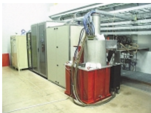
Figure 4. The complete modulator and klystron tank for the booster pre-injector.
