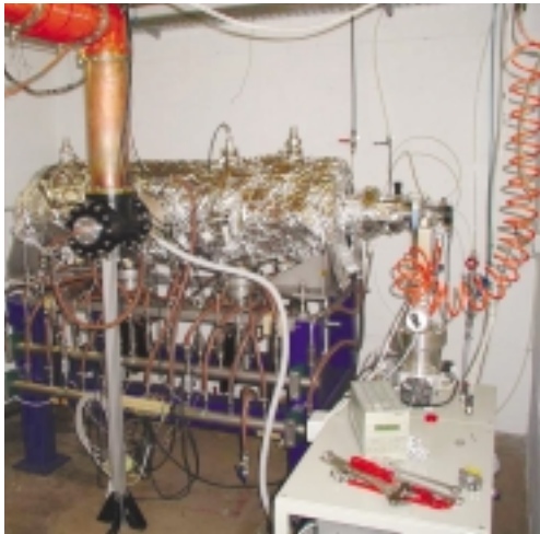
Figure 5. The five cell booster cavity undergoing power tests in the RF bunker.
