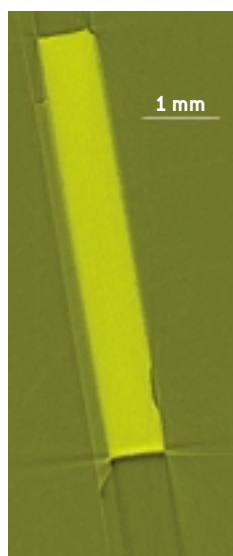
Figure 4. Reconstructed slice of a model glass covered by a thick organic polymer layer (Araldite®).
