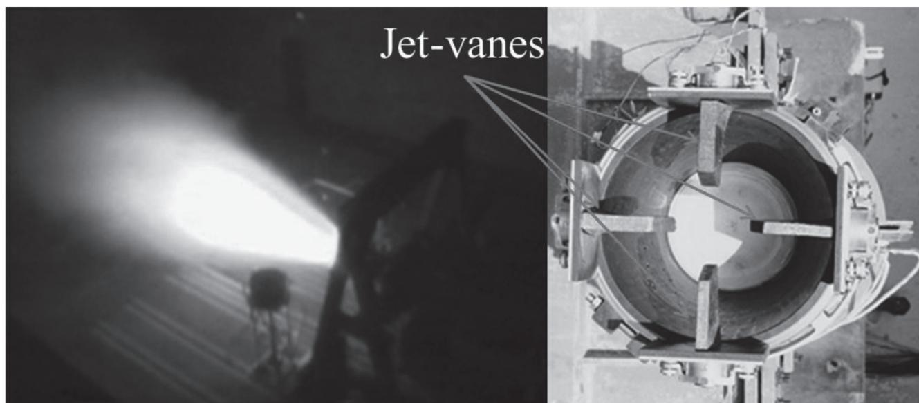
Fig. 3. Jet-vanes testing (static test)
