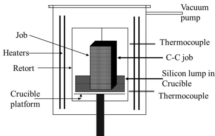
Fig. 1. Schematic of silicon infiltration
