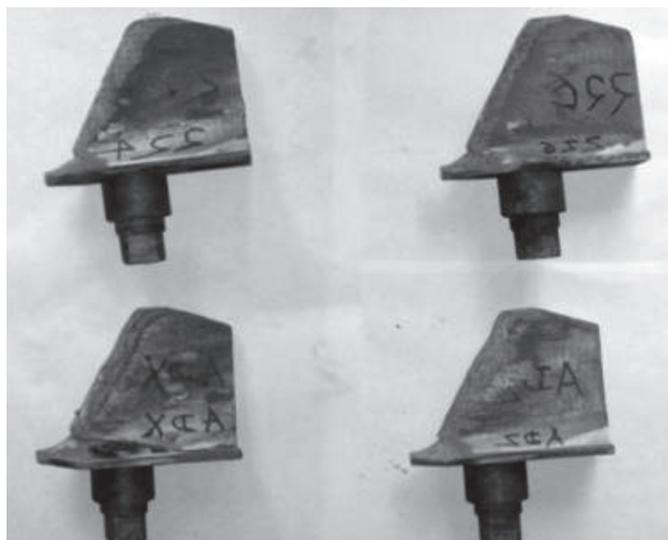
Fig. 4. Tested jet-vanes under rocket-motor exhaust
