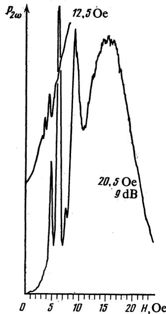
FIG. 2. Example of the recording of nonlinear resonances in indium ( $\mathbf{n} \parallel [011]$ ). The field  $\mathbf{H}$  in the plane of the sample makes an angle of  $40^\circ$  with the  $[100]$  axis,  $T = 3.4$  K). The curve with  $H_- = 12.5$  Oe is displaced upward.
