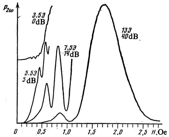
FIG. 1. Example of recordings of nonlinear resonances in bismuth ( $\mathbf{n} \parallel C_3$ ,  $\mathbf{H} \parallel C_1$ ,  $T = 1.5$  K). Near each of the curves is shown the value of  $H_-$  and the additional damping in the input attenuator of the detection system, in relative units. The curve with  $H_- = 3.5$  Oe is displaced upward.
