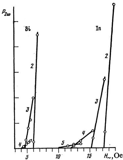
FIG. 3. Dependence of the amplitude of the resonance lines on  $H_{\sim}$  for bismuth and indium. Near the straight lines is shown the number  $n$  of the corresponding resonance.
