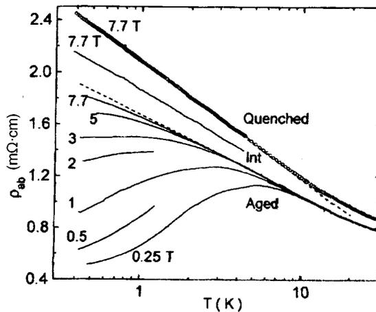
FIG. 1. In-plane resistivity versus  $\log T$  for a YBaCuO single crystal with a fixed oxygen content but with different oxygen arrangements (quenched, intermediate, and aged states). Only the aged state is superconducting, and the set of curves demonstrates how a field  $\mathbf{H}\parallel c$  destroys the superconductivity. The dashed lines are an extrapolation of the linear dependence  $\rho_{ab}(\log T)$ . Experimental points are plotted only on one curve.
