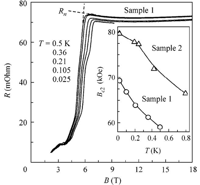
Fig. 3. The  $R(B)$  curves for sample 1 at temperatures (from left to right) from 0.5 K to 25 mK. Inset: the field of the onset of transition at low temperatures for both samples.
