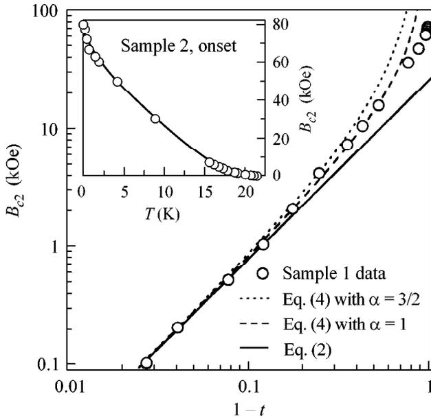
**Fig. 4.** Comparison of the experimental  $B_{c2}$  values for sample 1 with Eqs. (2) and (4). Inset: the  $B_{c2}(T)$  function for sample 2 over the entire temperature range. The line is a guide to the eye.
