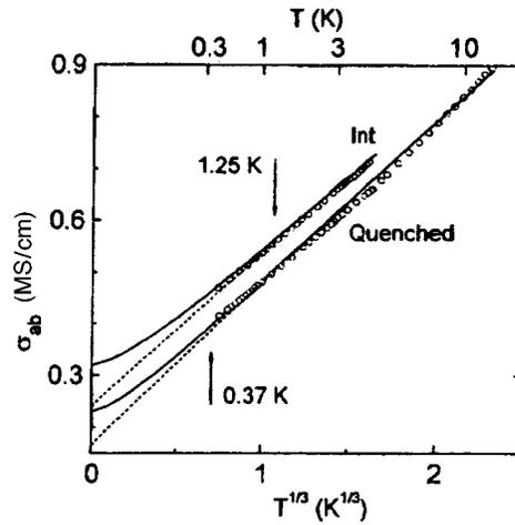
FIG. 2. The data for quenched and intermediate states from Fig. 1 replotted as  $\sigma_{ab}$  vs  $T^{1/3}$ . Solid lines – fits by Eq. (3) with the  $T^*$  values indicated by arrows, dashed lines – asymptotes in the  $t \gg 1$  region.
