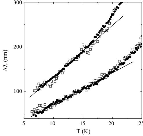
Fig. 3 – Comparison of  $\Delta\lambda(T)$  data at 9.4 GHz (black circles) and at 100 kHz (open squares) in  $\text{MgB}_2$  samples #1 and #2. The upper graph is shifted by 20 nm up for clarity.
