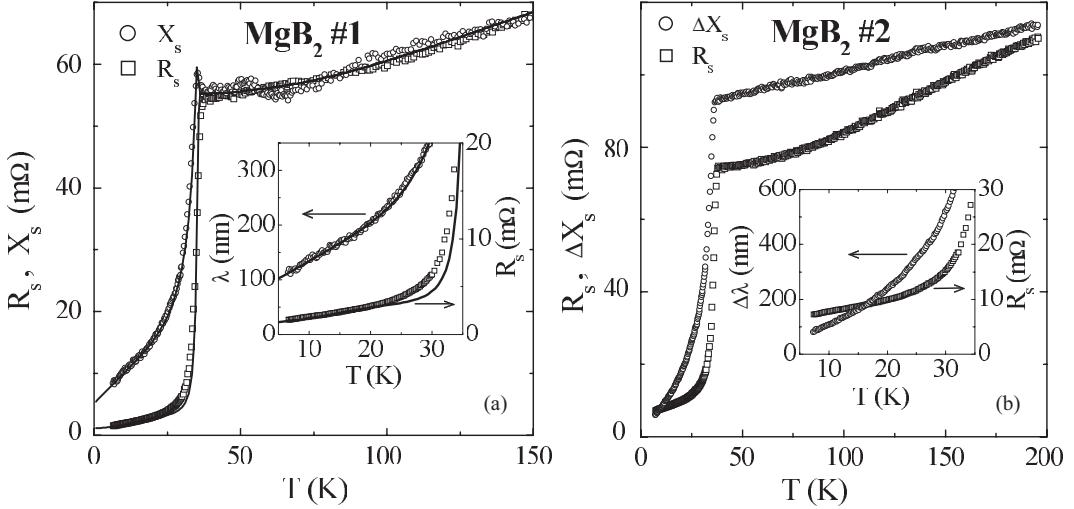
Fig. 2 – Plots of the surface resistance  $R_s(T)$  and reactance  $X_s(T)$  at 9.4 GHz in  $\text{MgB}_2$  samples #1 (a) and #2 (b). The insets show the low-temperature sections of  $R_s(T)$  and London penetration depth  $\lambda_L(T) = X_s(T)/\omega\mu_0$ . The solid curves in fig. 2(a) show calculations based on the modified two-fluid model.
