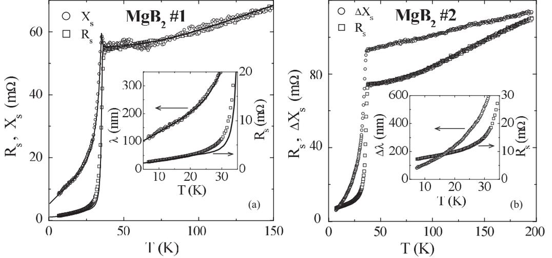
Fig. 2 – Plots of the surface resistance  $R_s(T)$  and reactance  $X_s(T)$  at 9.4 GHz in MgB<sub>2</sub> samples #1 (a) and #2 (b). The insets show the low-temperature sections of  $R_s(T)$  and London penetration depth  $\lambda_L(T) = X_s(T)/\omega\mu_0$ . The solid curves in fig. 2(a) show calculations based on the modified two-fluid model.
