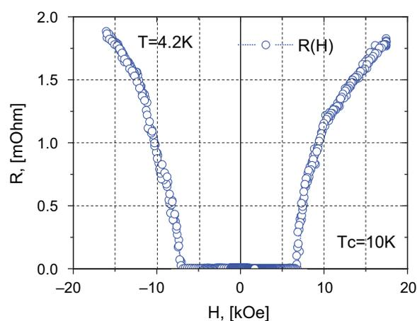
**Fig. 4.** Field dependence of resistance for Pb-Bi+Ce film.
