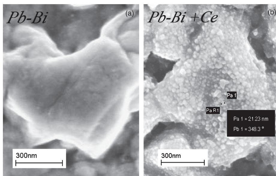
**Fig. 2.** The film surface (a) without Ce; (b) with Ce. The grain size around 20 nm.
