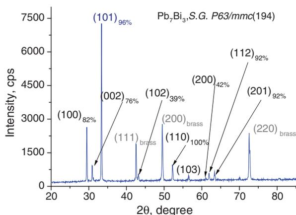
**Fig. 1.** The diffraction pattern of Pb/Bi-71/29 at.% film, grown on brass substrate by pulse electroplating. The percentages in the peaks indicate the intensity of the reflections.<sup>6</sup>
