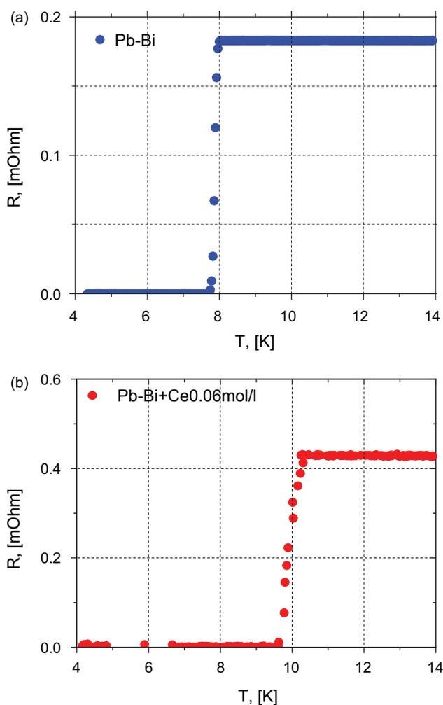
**Fig. 3.** (a) Temperature dependence of resistance for  $\text{Pb}_7\text{Bi}_3$  film. (b) Temperature dependence of resistance for Pb-Bi+Ce film.
