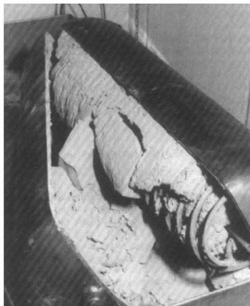
Fig. 36 – Left: layout of \text{MgH}_2 tank for a process steam generator. Right: The tank opened after 1.5 years of operation [345].
