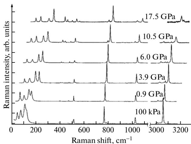
**Fig. 1.** Raman spectra of the naphthalene crystal at room temperature and pressures up to 17.5 GPa.
