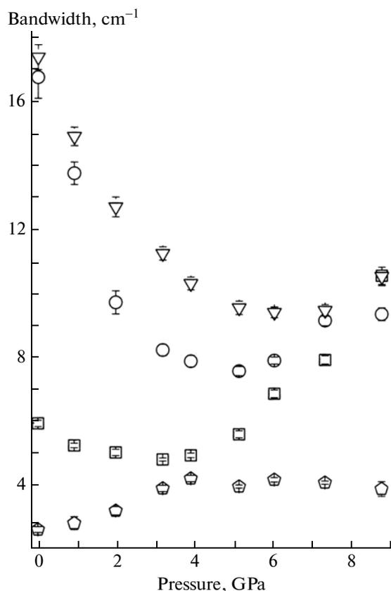
**Fig. 4.** Pressure dependence of the half-width of the phonon bands in the Raman spectrum of the naphthalene crystal at room temperature for phonons with frequencies of ( $\Delta$ ) 107, ( $\circ$ ) 123, ( $\square$ ) 3054, and ( $\diamond$ ) 1388  $\text{cm}^{-1}$ .
