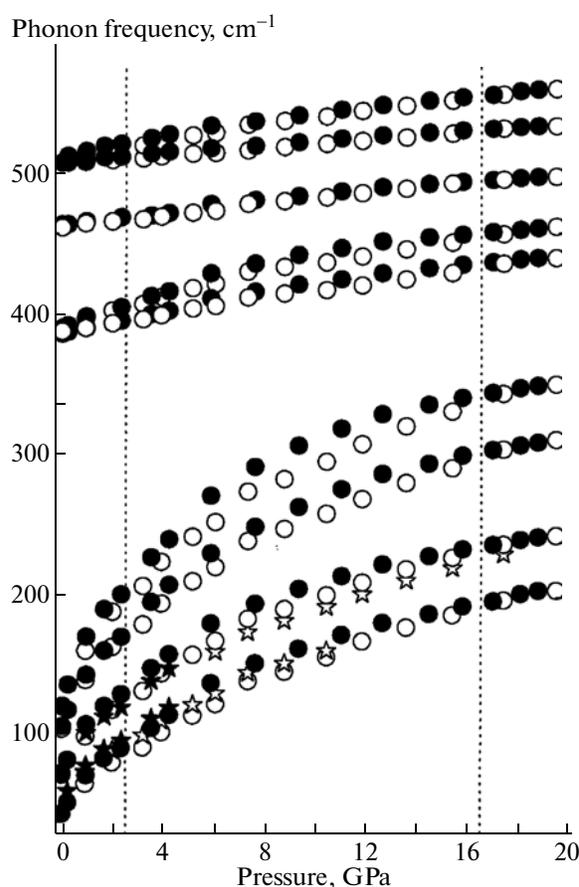
**Fig. 2.** Pressure dependence of the phonon frequency with an energy up to  $500\text{ cm}^{-1}$  in the naphthalene crystal at pressures up to  $20\text{ GPa}$ . Open and closed symbols correspond to the direct and inverse pressure variations, respectively. Asterisks indicate the frequencies of phonons that appear in the spectrum after the narrowing of the bands of intermolecular phonons at a high pressure.
