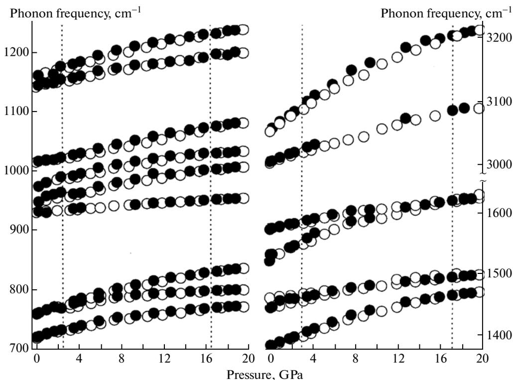
**Fig. 3.** Pressure dependence of the phonon frequency with an energy ranging from 700 to 3200  $\text{cm}^{-1}$  in the naphthalene crystal at pressures up to 20 GPa. Open and closed symbols correspond to the direct and inverse pressure variations, respectively.
