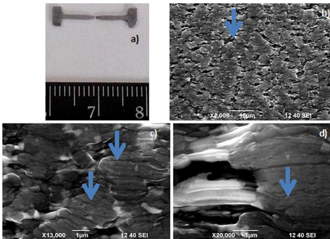
**Fig. 8.** (a) - sample view and (b, c, d) - deformation relief of the UFG Al–30Zn alloy after mechanical tensile tests at RT (SEM).
