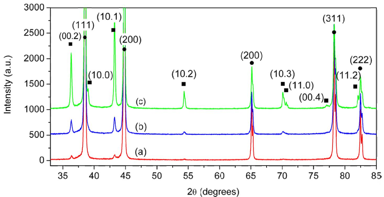
**Fig. 1.** Segments of X-ray patterns taken from Al alloys samples: (a) - Al-5Zn, (b) - Al-10Zn, (c) - Al-30Zn after HPT (● - Al; ■ - Zn).
