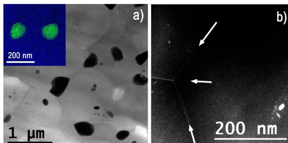
**Fig. 3.** UFG microstructure of Al-10Zn alloy after HPT: (a) - bright field STEM image and confirmed by the EDS map (inset, with Al-K blue and Zn-K green); (b) - dark field STEM image.
