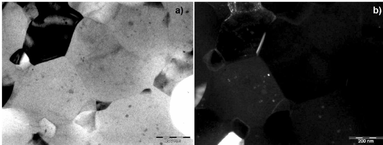
**Fig. 4.** UFG microstructure of Al-30Zn alloy after HPT: (a) - bright field TEM image; (b) - dark field TEM image.
