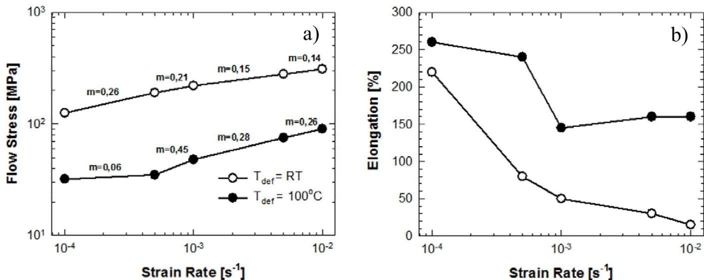
**Fig. 7.** Mechanical tensile tests of UFG samples of Al–30Zn alloy at RT (○) and at 100 °C (●): (a) - flow stress vs strain rate logarithmic dependence; (b) strain rate vs elongation to failure logarithmic dependence.
