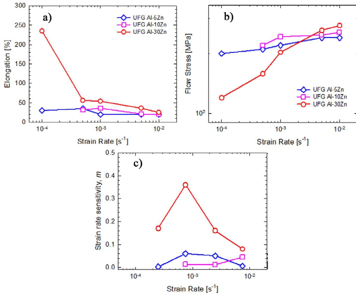
**Fig. 5.** Mechanical tensile tests of UFG samples of Al-5Zn, Al-10Zn, Al-30Zn alloys at RT: (a) - strain rate vs elongation to failure logarithmic dependence; (b) - flow stress vs strain rate logarithmic dependence; (c) - sensitivity coefficient (*m*) vs strain rate logarithmic dependence.
