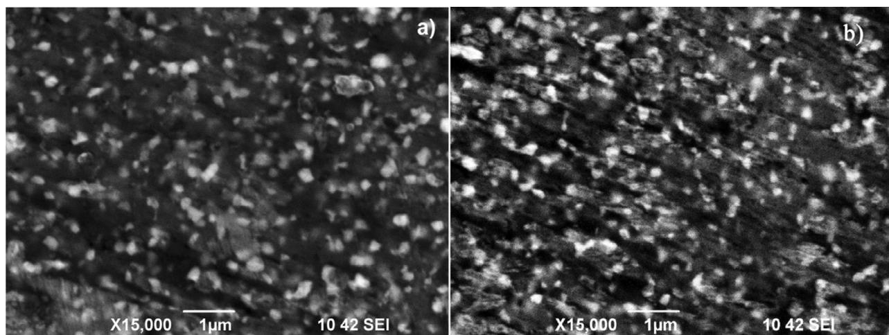
**Fig. 6.** Structure of UFG Al-30Zn alloy: (a) - before mechanical tensile tests; (b) - after mechanical tensile tests at RT (SEM).
