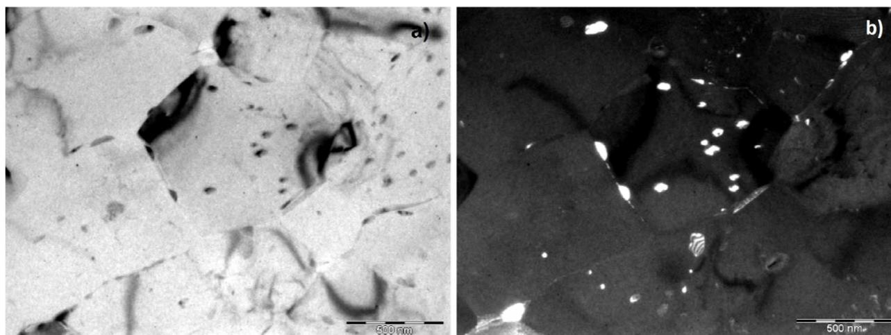
**Fig. 2.** UFG microstructure of Al-5Zn alloy after HPT: (a) - bright field TEM image; (b) - dark field TEM image.
