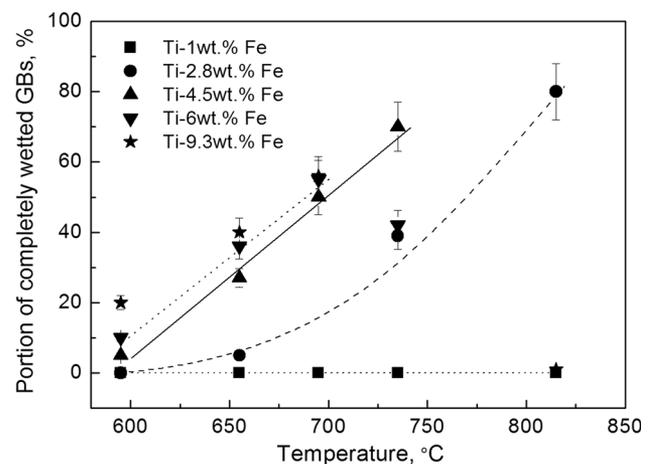
Fig. 4 Temperature dependence of the portion of completely wetted  $\beta(\text{Ti, Fe})/\beta(\text{Ti, Fe})$  GBs for Ti-1 wt.% Fe, Ti-2.8 wt.% Fe, Ti-4.3 wt.% Fe, Ti-6.5 wt.% Fe and Ti-9 wt.% Fe alloys
