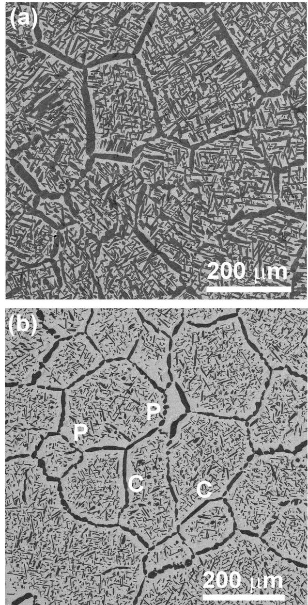
**Fig. 2** SEM micrographs of the Ti-4.5 wt.% Fe (a) and Ti-9 wt.% Fe (b) alloys annealed at temperature 695°C, 1032 h. The  $\alpha(\text{Ti, Fe})$  phase appears dark. The  $\beta(\text{Ti, Fe})$  phase appears bright. Letter C marks the  $\beta(\text{Ti, Fe})/\beta(\text{Ti, Fe})$  GBs completely wetted by the second solid phase  $\alpha(\text{Ti, Fe})$ . Letter P marks the  $\beta(\text{Ti, Fe})/\beta(\text{Ti, Fe})$  GBs partially wetted by the  $\alpha(\text{Ti, Fe})$  phase
