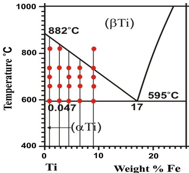
**Fig. 1** The part of the bulk phase diagram Ti-Fe. Vertical thin lines show the studied concentrations, and dots show the annealing temperatures
