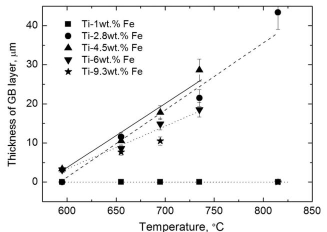
Fig. 5 Temperature dependence of the thickness of layer of  $\alpha(\text{Ti, Fe})$  phase in the  $\beta(\text{Ti, Fe})/\beta(\text{Ti, Fe})$  GBs for the Ti-1 wt.% Fe, Ti-2.8 wt.% Fe, Ti-4.3 wt.% Fe, Ti-6.5 wt.% Fe and Ti-9 wt.% Fe alloys
