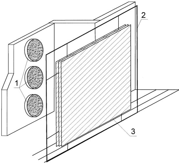
Fig. 1. Scheme of the industrial configuration for glass decorative coating: (1) Metallic cathodes, (2) mobile frame, (3) glass sheets mounted back to back.
