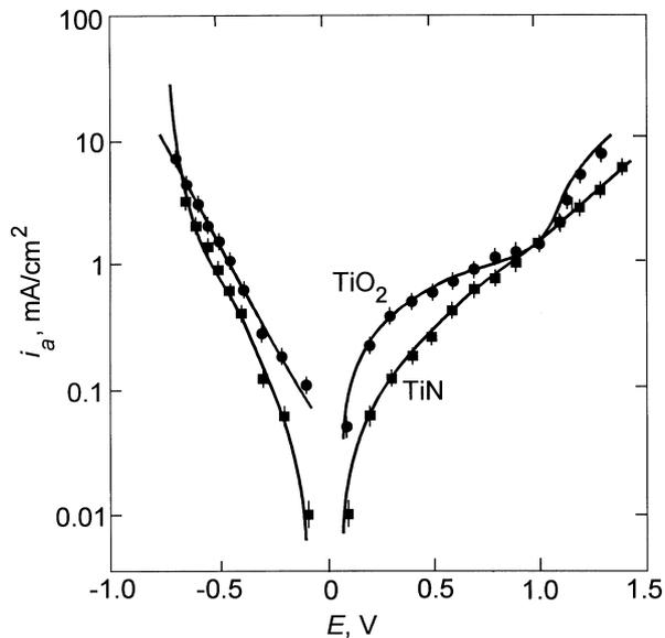
Fig. 4. Dependence of the anodic current  $i_a$  on the polarization voltage  $E$  for  $\text{TiO}_2$  and  $\text{TiN}$  coatings on silica glass in  $\text{NaCl}$  solution at  $\text{pH} = 7$ . The experimental points are connected with the guidelines for the eye. The error bars correspond to the standard deviation of the measurements.
