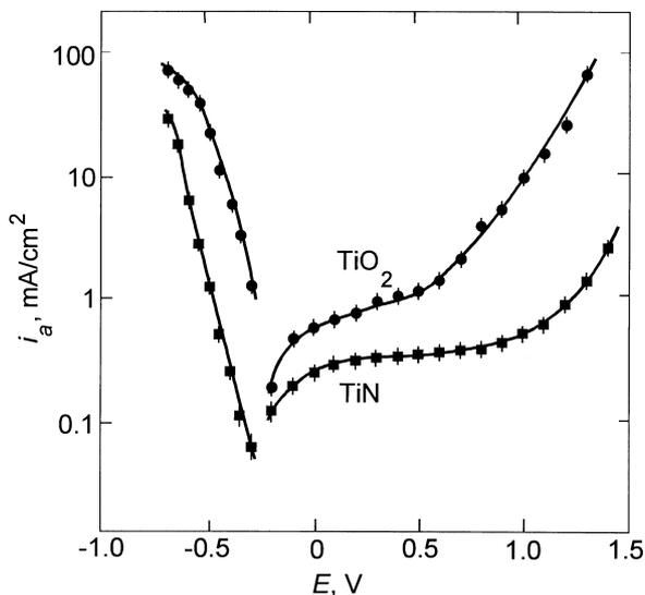
Fig. 5. Dependence of the anodic current  $i_a$  on the polarization voltage  $E$  for  $\text{TiO}_2$  and  $\text{TiN}$  coatings on silica glass in  $\text{NaCl}$  solution at  $\text{pH} = 3$ . The experimental points are connected with the guidelines for the eye. The error bars correspond to the standard deviation of the measurements.
