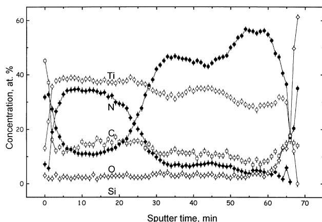
Fig. 3. AES depth profile for TiN/TiO<sub>2</sub> bilayer coating on silica glass. The experimental points are connected with the guidelines for the eye. The bars correspond to the statistical error of the spectrometer counting.
