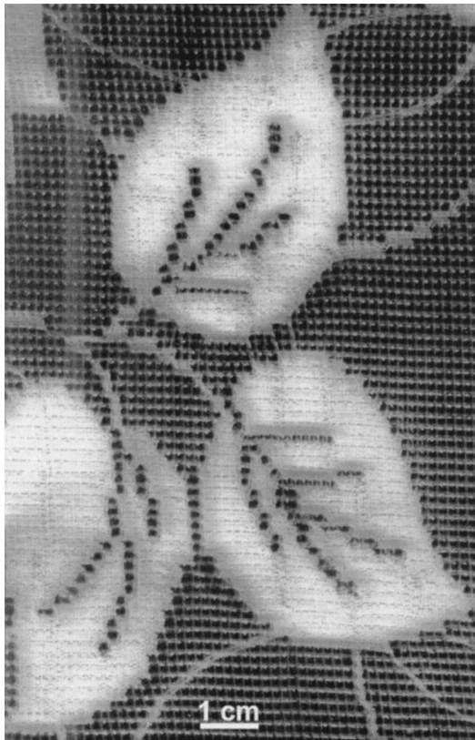
Fig. 2. Detail of a decorative pattern obtained by masking during TiN arc deposition on silica glass.
