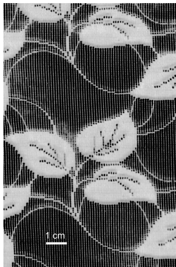
Fig. 1. Detail of a decorative pattern obtained by masking during TiN arc deposition on silicate glass.
