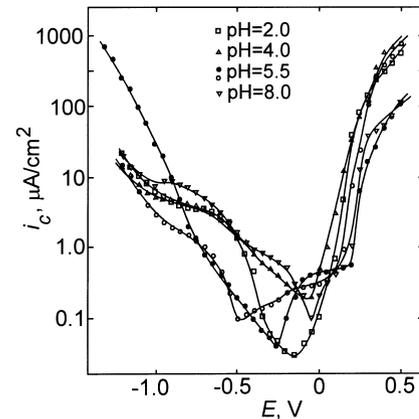
Fig. 4. The dependence of the corrosion current  $i_c$  on the polarisation voltage  $E$  in 3.0 at.% NH<sub>4</sub>Cl solution at various pH values for H18N10T stainless steel vacuum arc coated with a TiN layer (open symbols) and uncoated (full symbols). The lines are guides for the eye.
