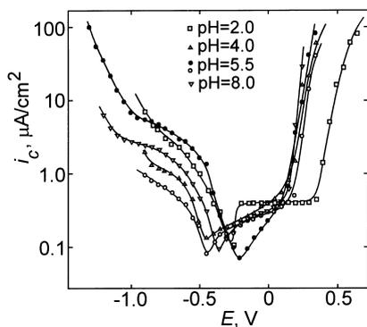
Fig. 3. The dependence of the corrosion current  $i_c$  on the polarisation voltage  $E$  in 3.0 at.% NaCl solution at various pH values for H18N10T stainless steel vacuum arc coated with a TiN layer (open symbols) and uncoated (full symbols). The lines are guides for the eye.
