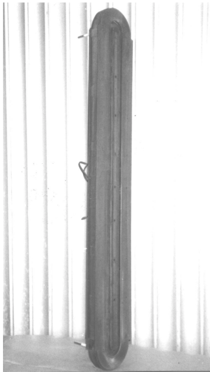
Fig. 1. Hall current accelerator. The total length (aperture) is 1400 mm.
