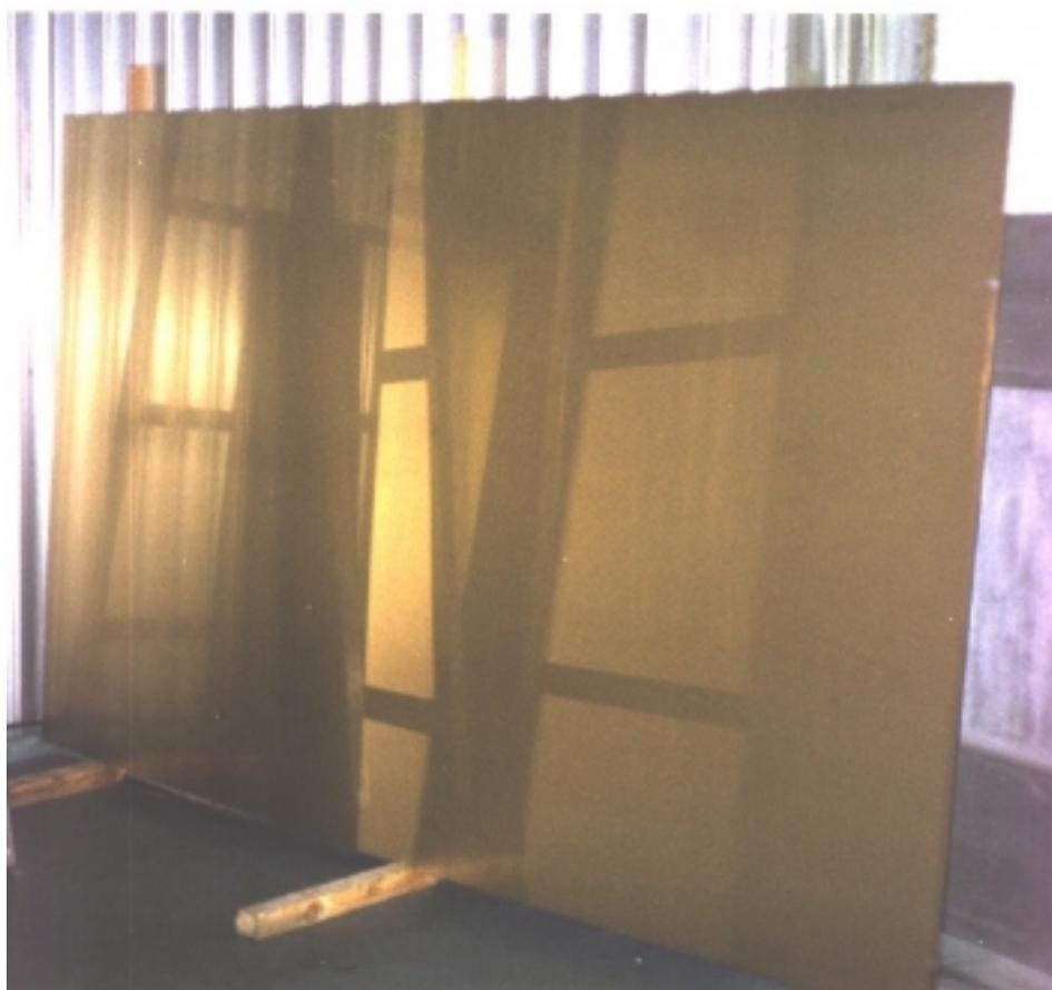
Fig. 4 The individual element (1×2 m TiN coated stainless steel strip) of the new roof for the Moscow Luzhniki Olympic Stadion.
