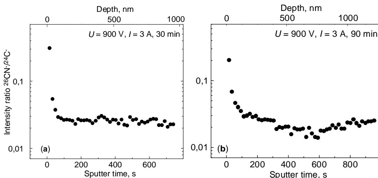
Fig. 5. SIMS depth profiles for the nitrogen implanted into stainless steel at  $U = 900 \text{ V}$  and  $I = 3 \text{ A}$ . Implantation time  $t = 30 \text{ min}$  (a) and  $90 \text{ min}$  (b).
