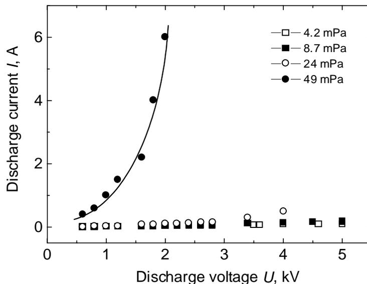
Fig. 2. Current-voltage characteristic for nitrogen at various pressures.
