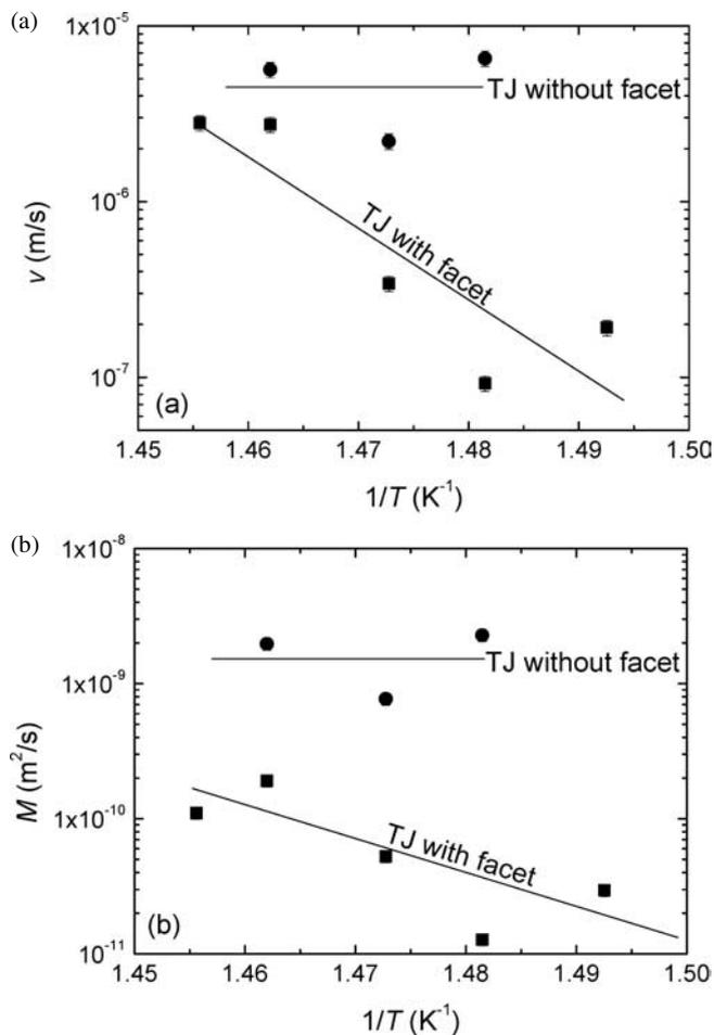
Fig. 6. (a) Temperature dependence of the migration rate  $v$  and (b) mobility  $M$  of TJs with rough (circles) and faceted GBs (squares) in Arrhenius coordinates.
