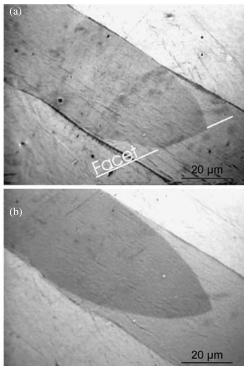
Fig. 2. Micrographs of the TJ obtained in an *in-situ* hot-stage experiment at 679 K using polarized light. Two typical shapes are shown for: (a) with facet in GB with misorientation angle  $37^\circ$  and (b) without facet.
