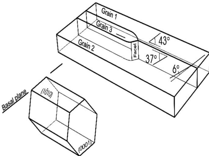
Fig. 1. Scheme of the Zn tricrystal containing three  $[10\bar{1}0]$  tilt GBs with misorientation angles of  $43^\circ$  (between grain 1 and grain 3),  $37^\circ$  (between grain 2 and grain 3), and  $6^\circ$  (between grain 1 and grain 2). The orientation of the basal plane (0001) is shown in all three grains. The facet formed in the GB with misorientation angle  $37^\circ$  is also shown.
