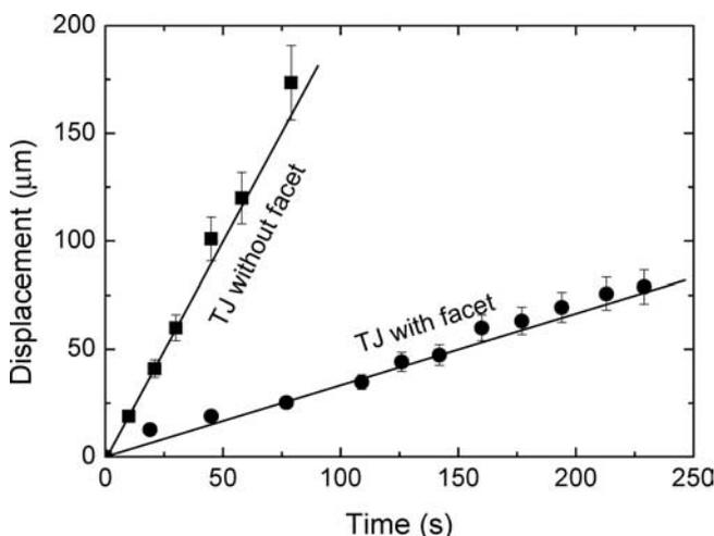
Fig. 3. Time dependence of TJ displacement for a TJ with facet and without facet (679 K).
