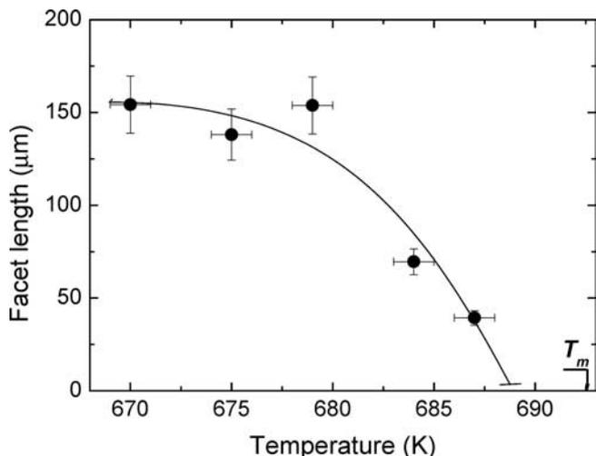
Fig. 5. Temperature dependence of the facet length in the  $\theta = 37^\circ$  GB.
