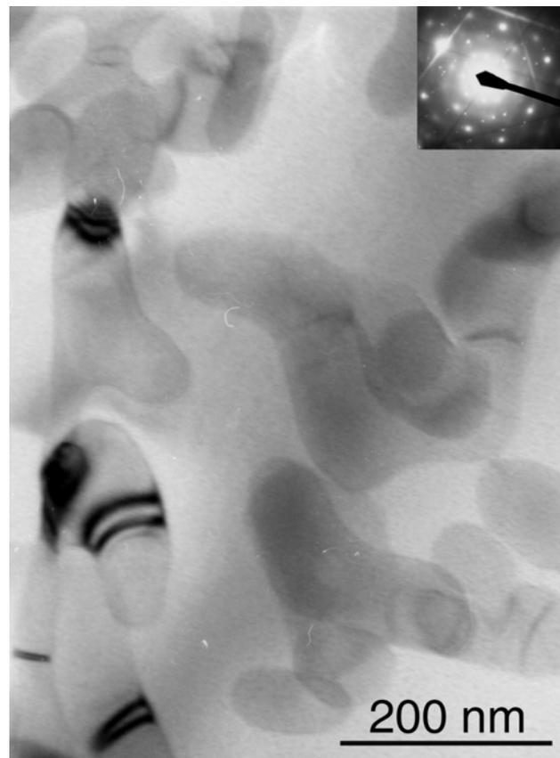
Fig. 1b Microstructure of coarse grained Al–10%Zn–4%Mg alloys (as cast state)
