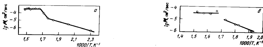
Figure 9. Temperature dependencies of the mobility of tilt GB \langle 11\bar{2}0 \rangle in zinc.
