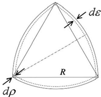
Fig. 2. Diagram of a 3-sided grain with an inscribed equilateral triangle with sides of length  $R$ . Each boundary of the grain is an arc of a circle and the internal dihedral angle at each corner is 120°, corresponding to local vertex equilibrium and isotropic grain boundary energy. If the grain shrinks in size by  $dR$  each vertex of the inscribed triangle moves in by  $d\rho$  and each boundary arc moves in by  $d\varepsilon$ , where  $dR = d\varepsilon + d\rho$ .
