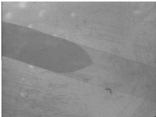
Fig. 4. Grain boundary with the “rough-to-rough” ridge of first-order at the half-loop ( $T = 345\text{ °C}$ ).
