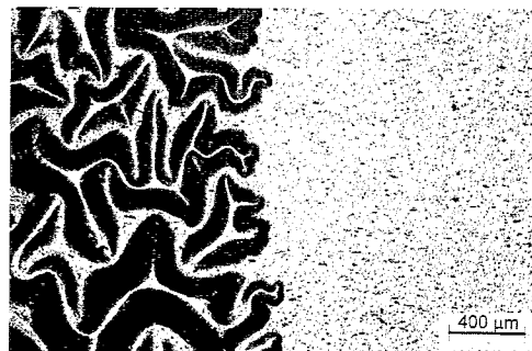
Fig. 3. Optical micrograph of the microstructure of the Mo coating on silica glass ( P = 4.3 kW, L = 50 mm, t = 5 min, \theta = 0^\circ , d = 0.5 \mu\text{m} ). A part of the coating delaminates spontaneously from the substrate (see left side of the micrograph).
