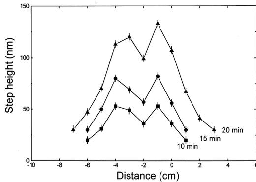
Fig. 3. Source cleaning profile for silica glass. The experimental points are connected with the guidelines for the eye.
