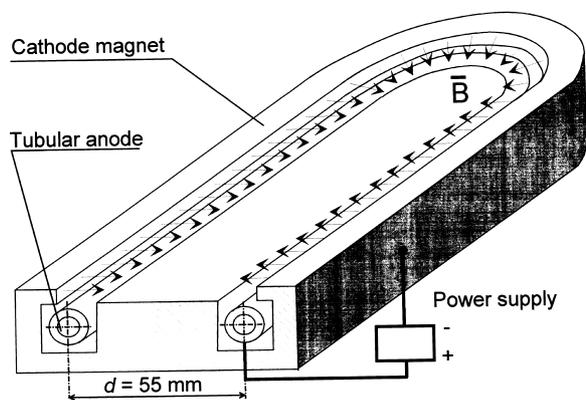
Fig. 1. Hall current accelerator half view.
