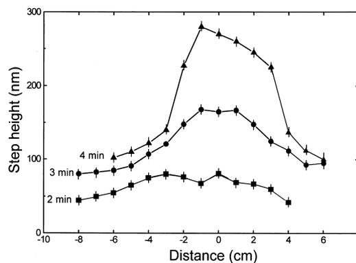
Fig. 2. Source cleaning profile for poly(methyl metacrylate). The experimental points are connected with the guidelines for the eye.
