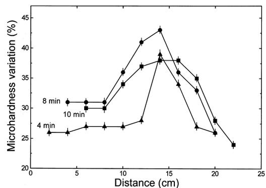
Fig. 4. Source cleaning profile in terms of microhardness variation for Al alloy 5182. The experimental points are connected with the guidelines for the eye.
