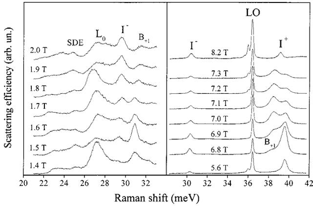
FIG. 1. Inelastic light scattering spectra of a sample with a QW width of 250 Å and  $n_s = 6.8 \times 10^{11} \text{ cm}^{-2}$  measured at  $q = 1.1 \times 10^5 \text{ cm}^{-1}$ ,  $E_L = 1.59 \text{ eV}$ , and magnetic fields where resonances between  $\text{ISBM}_{+1}$  and  $I^-$  (left), and  $\text{ISBM}_{+1}$  and  $I^+$  (right) occur.
