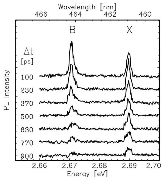
FIG. 1. Transient PL spectra of one single CdSe/ZnSe quantum dot including single exciton ( $X$ ) and biexciton ( $B$ ) emission. The excitation flux was  $\Phi = 4.0 \mu\text{J cm}^{-2}$ .
