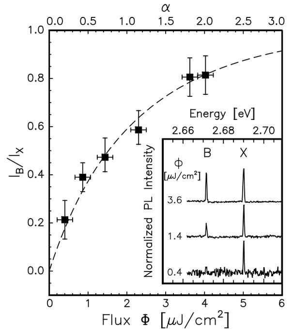
FIG. 3. Ratio of the time-integrated intensity  $I_B/I_X$  as a function of the excitation flux  $\Phi$ . Experiment: symbols; theory according to Eqs. (2): dashed line. In the inset, time-integrated PL spectra are depicted for different  $\Phi$ .
