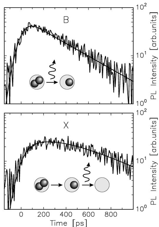
FIG. 2. Decay characteristics of the single exciton ( $X$ ) and the biexciton ( $B$ ) transition. The solid lines represent model calculations as discussed in the text.
