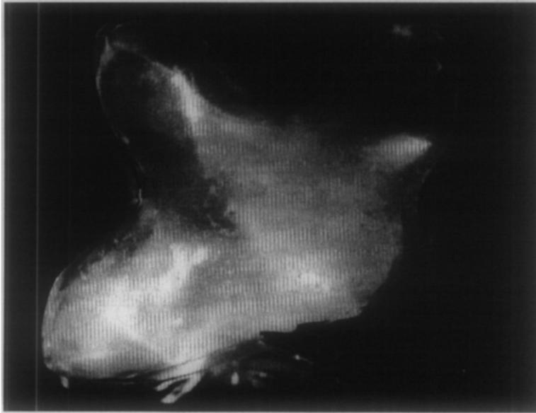
Fig. 9. Cross-section of a  $Gd_2(MoO_4)_3$  crystal grown by the conventional Czochralski technique in the [001] direction.
