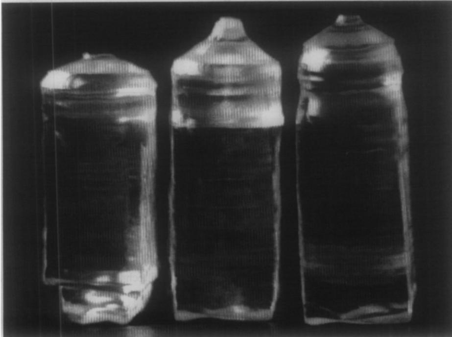
Fig. 11. Gadolinium molybdate crystals with a maximum transverse cross-section of 30 mm grown with use of modified Czochralski technique.
