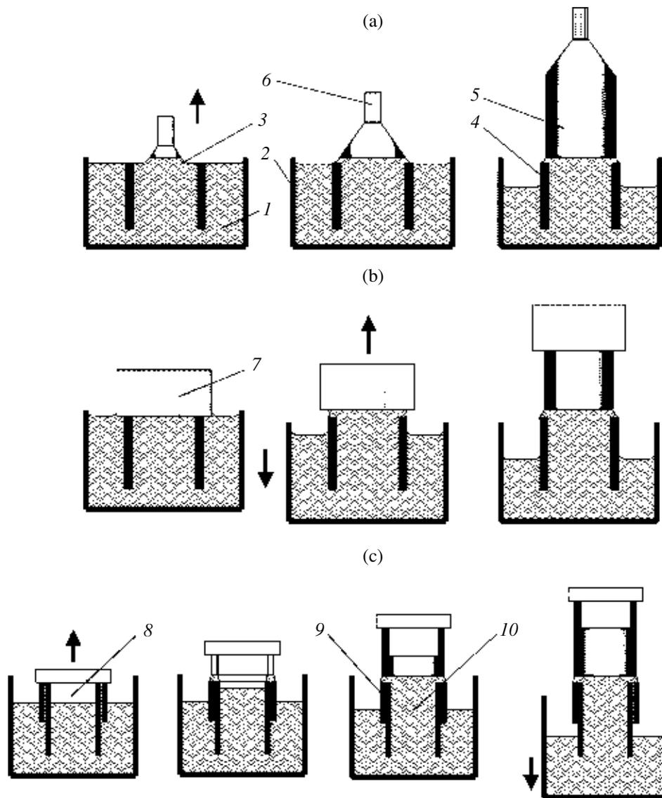
**Fig. 4.** Schematic picture illustrating the growth of shaped bulk crystals by the NCS technique: (a) with the use of pointlike seed; (b) with the use of bulk seed; (c) with the use of a capillary channel; (1) melt; (2) crucible; (3) meniscus; (4) shaper; (5) crystal; (6) pointlike seed; (7) bulk seed; (8) closed volume under the seeding plate; (9) capillary channel; (10) noncapillary channel.
