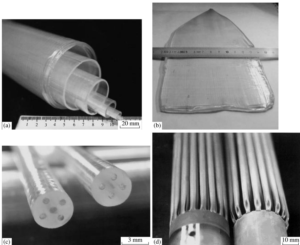
**Fig. 2.** The shaped crystals grown by the Stepanov method (EFG with the weight control): (a) tube up to 85 mm in diameter; (b) tape 120 mm wide; (c) bar with channels 0.7 mm in diameter; (d) bars and tubes grown in the group mode.
