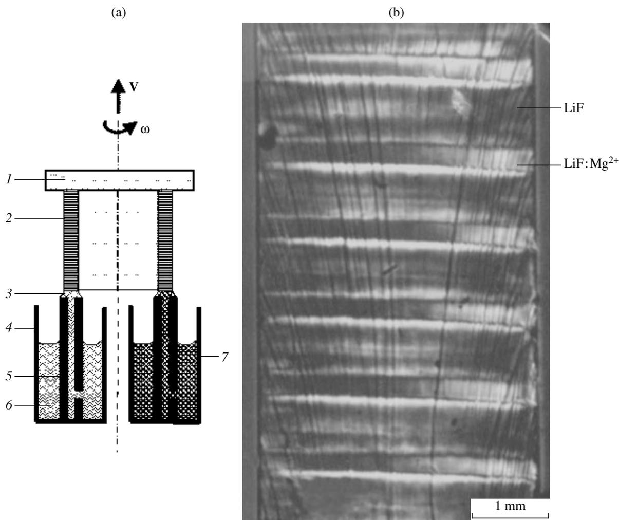
**Fig. 8.** Manufacturing of periodic structures by the GES technique: (a) layout of the growth setup ((1) seed; (2) crystal with the periodic structure; (3) melt meniscus; (4) crucible; (5) shaper; (6) undoped melt; (7) doped melt); (b) LiF–LiF:Mg<sup>2+</sup> crystal with the periodic structure (the photo is taken in polarized light).
