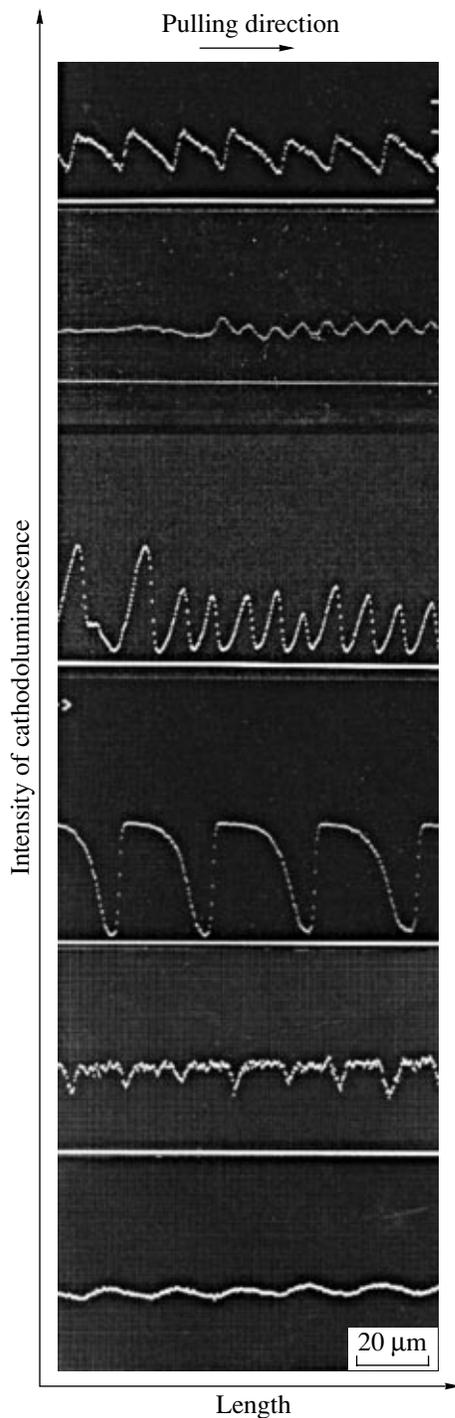
**Fig. 10.** The intensity distribution for the cathodoluminescence corresponding to the content of the luminescent impurity for different kinds of  $\text{Al}_2\text{O}_3\text{-Al}_2\text{O}_3\text{:Ti}^{3+}$  structures produced by the GES technique.
