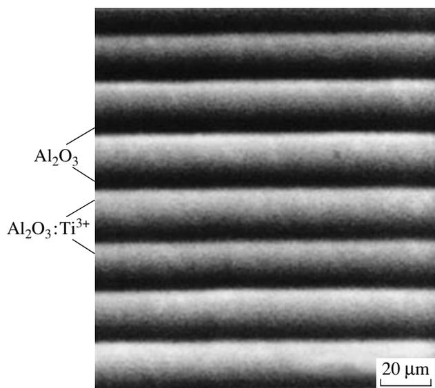
**Fig. 9.** Periodic Al<sub>2</sub>O<sub>3</sub>–Al<sub>2</sub>O<sub>3</sub>:Ti<sup>3+</sup> structure produced by the GES technique.
