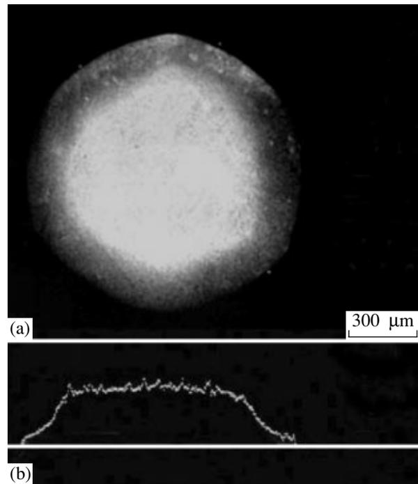
**Fig. 11.** (a) The cross section of an  $\text{Al}_2\text{O}_3\text{-Al}_2\text{O}_3\text{:Ti}^{3+}$  filament grown with the use of the weight control system and (b) the corresponding intensity distribution for the cathodoluminescence.
