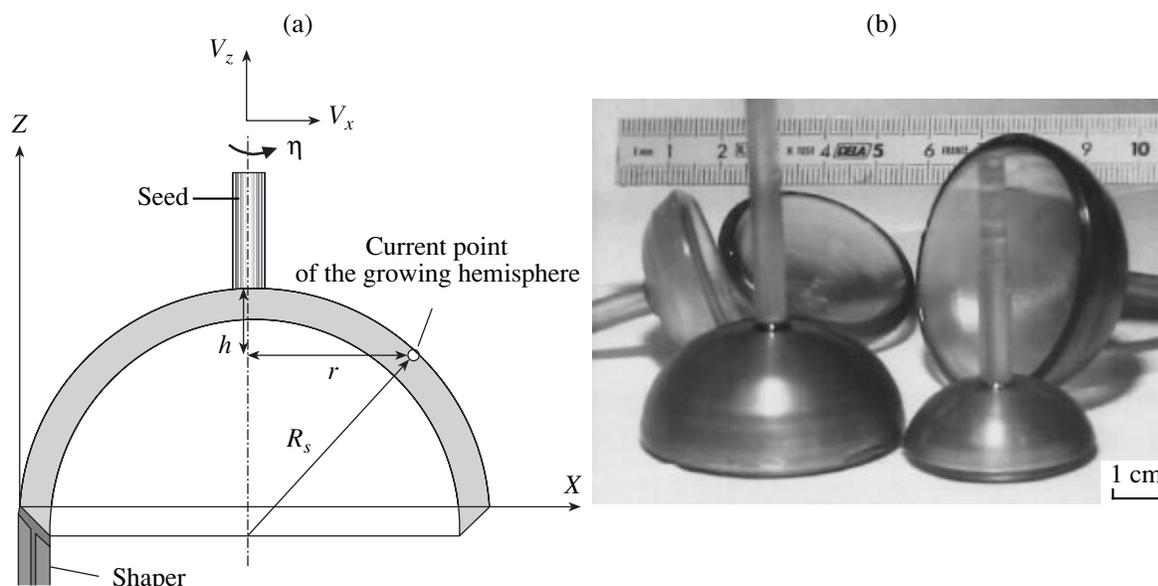
**Fig. 7.** The growth of hemispheres by the GES technique: (a) the growth scheme using the shaper with an inclined end face; (b) photos of sapphire hemispheres up to 50 mm in diameter with walls up to 4 mm thick.
