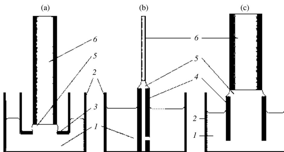
**Fig. 1.** The layout of different versions of the Stepanov method: (a) the classical version with the use of the shaper not wetted by the melt; (b) the EFG method; (c) the method with the use of the noncapillary feeding; (1) melt; (2) crucible; (3) shaper not wetted by the melt; (4) shaper wetted by the melt; (5) meniscus; (6) crystal.
