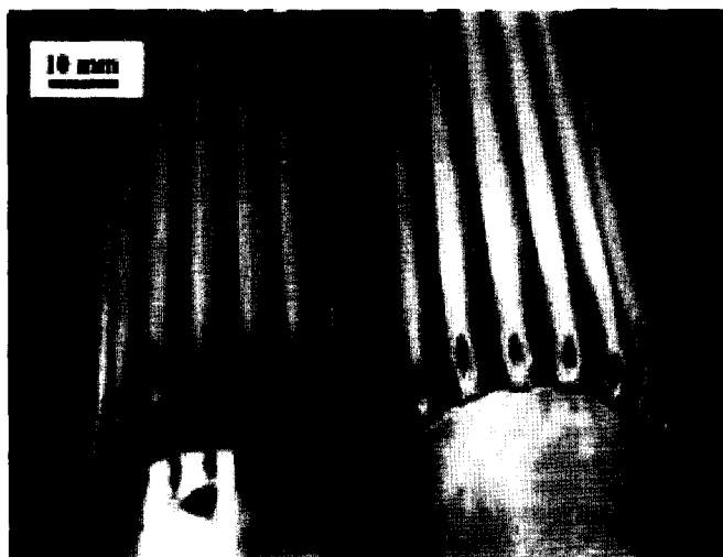
Fig. 40. Sapphire crystals grown by multi-run pulling process (rods 3.0 mm in diameter and tubes 3.5 mm in outer diameter).
